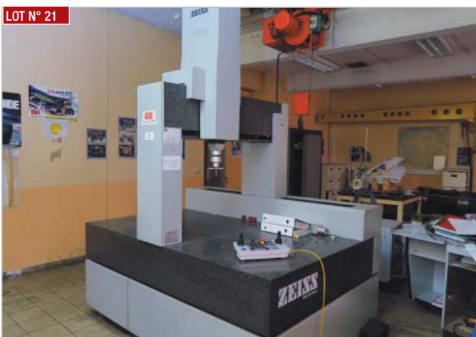
▶ Machine à mesurer tridimensionnelle ZEISS MC 850 , Marbre granit 2100 x 1400, Entre portique = 1000mm, Hauteur = 500mm ▶ Three-dimensional measuring machine ZEISS MC 850, Granite marble table 2100 x 1400, Gantry width = 1000mm, Height = 500mm
